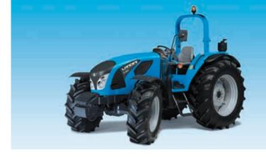
Three years after its launch in 2012, the 5H tractor range is now revamped with a newly redesigned cab. Featuring a four-post design with flat-deck platform and rear hinged doors, the new cab provides ease of access to the driver's seat and unequalled allround visibility.
