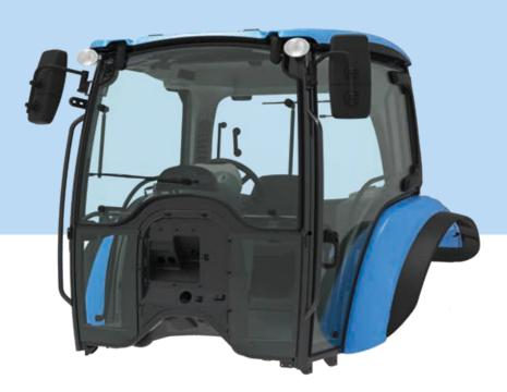
easy manoeuvring in tight spots, while the transparent roof hatch provides extra visibility for front loader operations. The Total View Slim cab meets FOPS (Falling Objects Protecting Structure) safety standards for the use of front-end loaders. The cab is also available with rear narrow fenders which, combined with a suitable tyre size, allow the **4 Series** tractor to achieve a minimum width of only 1750 mm, making it ideal for working between tight orchard and vineyard rows.
