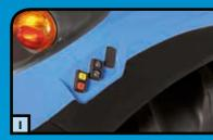
Exernal PTO and hitch controls are located on the rear fenders, making it easier to attach implements from the ground (fig. I).
