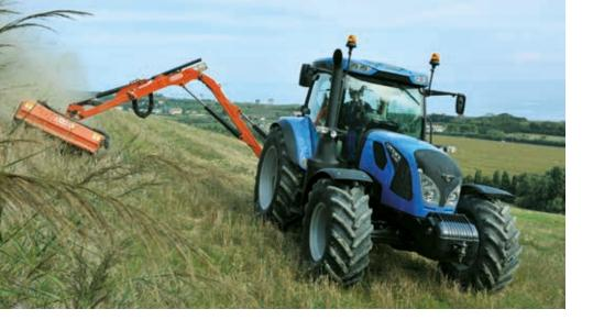
The new 6C series comprises three models, all powered by the new FPT-NEF 4.5L engines with power ratings of 114, 121 and 130 hp. All engines meet the Tier 4 Final emission standards using a new after-treatment technology that combines a selective catalytic reduction system (SCR) and a diesel oxidation catalyst (DOC). In addition, they feature the Dual Power system which boosts engine power to 121, 133 and 140 hp, respectively, for PTO and transport applications.
