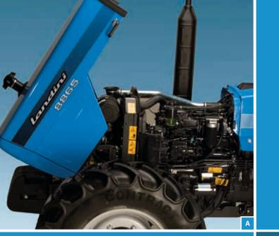
8865 models) are equipped with the new environment-friendly Perkins 1104C 4-cylinders engines. The new engines deliver 75 and 81.6 HP (ISO) respectively, while offering high torque backup, improved fuel economy, low noise and
