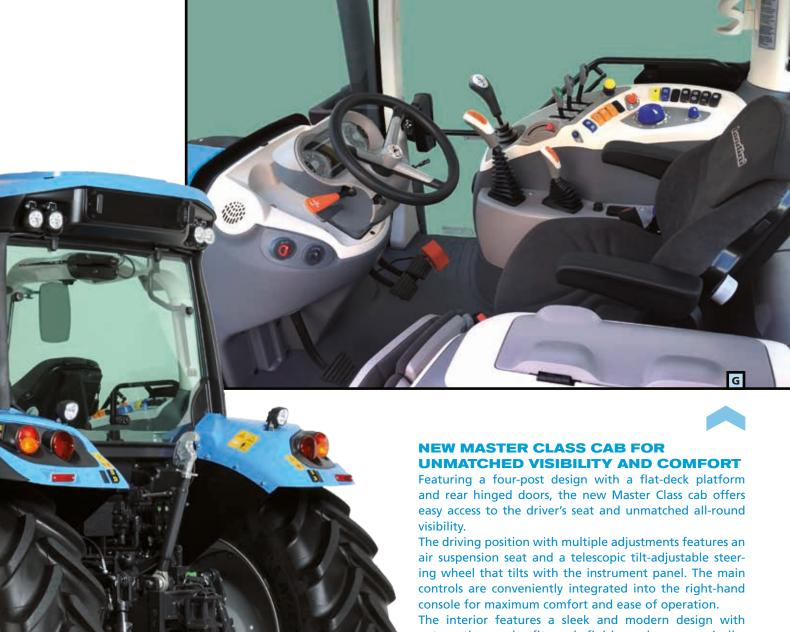
The interior features a sleek and modern design with automotive-grade fit and finish and ergonomically-arranged controls. Perfectly sound-proofed, pressurised and air-conditioned, the cab of the 6C tractor offers a comfortable environment for long hours in the field.
