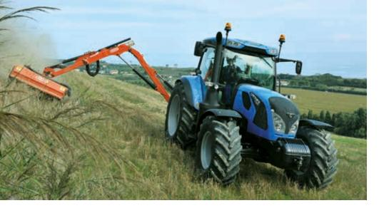
The new 6C Series from Landini is the successor to the popular Powermondial tractor family. The three models in the range are powered by the new FPT NEF 4.5L engines with power ratings of 114, 121 and 133 hp.
