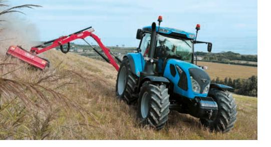
The new 6C series comprises three models, all powered by the new FPT-NEF 4.5L engines with power ratings of 114, 121 and 130 hp. All engines meet the Tier 4 Final emission standards using a new after-treatment technology that combines a selective catalytic reduction system (SCR) and a diesel oxidation catalyst (DOC). In addition, they feature the Dual Power system which boosts engine power to 121, 133 and 140 hp, respectively, for PTO and transport applications.
