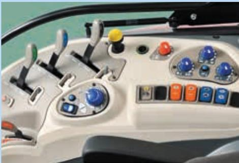
The **6H** can be equipped with up to four remote valves. Three valves are mechanically operated by levers and one is controlled electro-hydraulically via a pushbutton. Two additional mid-mount remotes are available as an option for the use of L Series front loaders or other front-mounted implements.
