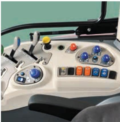
The electronically-controlled rear hitch features ergonomically-designed easy-to-use controls and is equipped with lower link draft sensing for precise implement control. The three-point hitch is Category II and offers a maximum lift capacity of 6000 kg. External hitch controls are located on the rear fenders making it easier to attach implements from the ground. The **6H** tractors are equipped with a hitch dampening function to prevent pitching when travelling with hitch-mounted implement.
