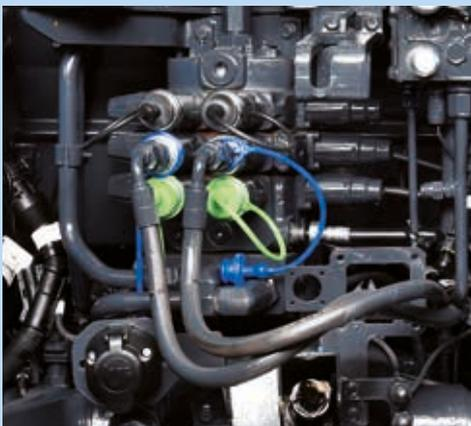
Each option allows the tractor to work with the front hitch, the front loader, the rear hitch and a variety of front- and rear-mounted implements for maximum efficiency and productivity. High-quality quick-release couplings, conveniently fitted on both the front and rear of the tractor, allow quick and easy connection/disconnection of hydraulic lines for fast operation.
