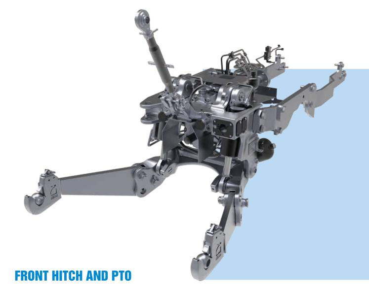
A front hitch and PTO are available as an option to add greater versatility to the **5 Series** tractor for applications using rearand front-mounted implement combinations. Offering a maximum lift capacity of 2200 kg, the front hitch is Category II and features raise/lower and float controls. The 1000-rpm PTO is engaged via a pushbutton. External PTO and hitch controls are also located on the rear fenders making it easier to attach implements from the ground.
