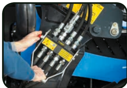
Quick-connect multi-coupler for tractor/loader hydraulic connection
