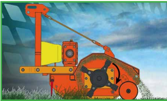
Clockwise rotation of belt driven hammer roller deposit cuttings behind adjustable 194mm diameter support roller.
