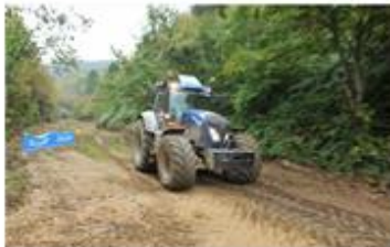
Landini 130 Hours Endurance 10.jpg Fast but bumpy forest tracks were a good test of operator comfort – a good air seat, cab suspension and independent front axle suspension all help.
