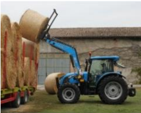
Landini 5-110H T4i + Landini MC80 loader 02.jpg A 113hp Landini 5-110H with the new MClassic 80 mechanical levelling loader.
