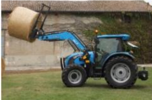
Landini 5-110H T4i + Landini MC80 loader 01.jpg A 113hp Landini 5-110H with the new MClassic 80 mechanical levelling loader.
