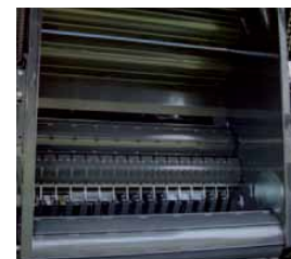
PowerMax Chamber: 17 heavy duty rollers for high density bale production.
