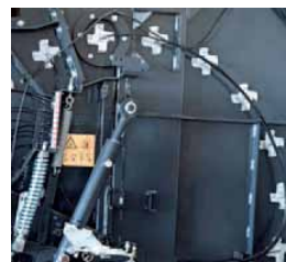
All rollers are carried on heavy duty, greasable bearings. Bearings are easily serviced from centralized greasing banks.
