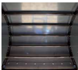
The bale chamber concept consists of 5 or 7 rollers, depending on model, at the front...
