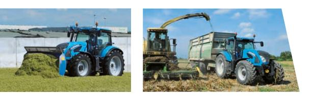
The 7 SERIES LANDINI Tier 4 Final: equipped with new 6-cylinder FPT - NEF Tier 4 Final engines, this series features a 2,820 mm standardized wheelbase.
