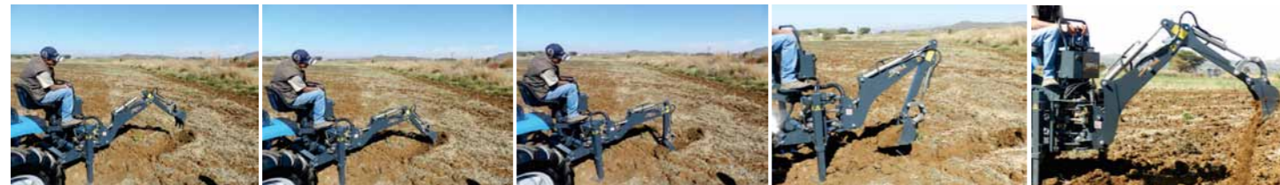
Hydraulic cylinders control all backhoe movements and allow boom swing of 180°.
