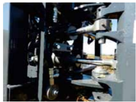
Hydraulic cylinders control all backhoe movements and allow boom swing of 180°.
