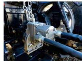
Backhoe hydraulic pump driven by the tractor PTO.
