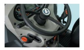
**SYNCHRO SHUTTLE** The **REX3** offers standard a synchro shuttle with control lever adjacent to the steeering wheel.
