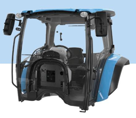
in tight spots, while the transparent roof hatch provides extra visibility for front loader operation. The Total View Slim cab meets FOPS (*Falling Objects Protecting Structure*) safety standards for the use of front-end loaders. Fitted with a suitable tire size, the Serie 4 tractor reaches a minimum width of only 1820 mm, making it ideal for working between wide vineyard and orchard rows.
