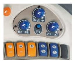
A front hitch and PTO are available as an option to add greater versatility to the Serie 5 tractor for applications using rear- and front-mounted implement combinations. Offering a maximum lift capacity of 2200 kg, the front hitch is Category II and features raise/lower and float controls. The 1000-rpm PTO with wet multi disc clutch is engaged electro-hydraulically. PTO controls are located both inside the cab and on the rear fenders making it easier to attach implements from the ground.
