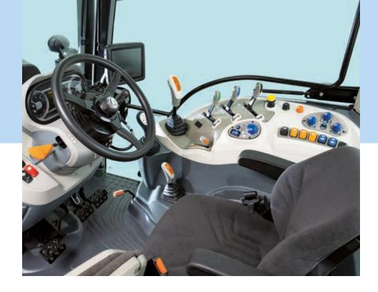
The four-post cab design with its all-round glazing provides unobstructed view in every direction, making manoeuvring in tight spaces and at headlands easier and safer, while a transparent roof hatch provides extra visibility for loader operation. Up to 10 LED work lights ensure optimum illumination of the working area at night.
