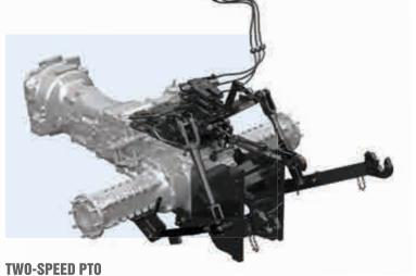
The Serie 4 features a rear 540/540E PTO with ground speed. A push button enables smooth and modulated engagement of the PTO, ensuring a soft start-up of the implement.
