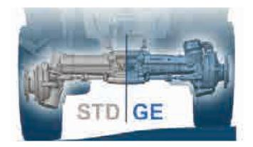
**MISTRAL2 GE, SPECIALISED IN LOW-CLEARANCE OPERATIONS** Specially designed for work in vegetable growing farms, greenhouses, vineyards and orchards grown on overhead trellis systems, the Mistral2 comes fitted with 20" and 24" rear tyres for maximum traction and stability. The front and rear axles of the Mistral2 GE are respectively 100 mm and 95 mm lower than on the Mistral2 STD.
