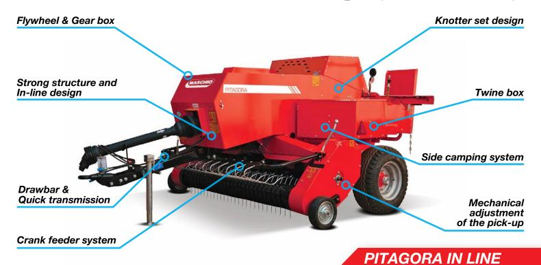
Enhance productivity with the IN-LINE baler: the high speed plunger 105 strokes/minute and the pick-up design offer best-in-class performance. The IN-LINE baling flow ensure perfectly shaped bales that can easily be collected with an accumulator.
