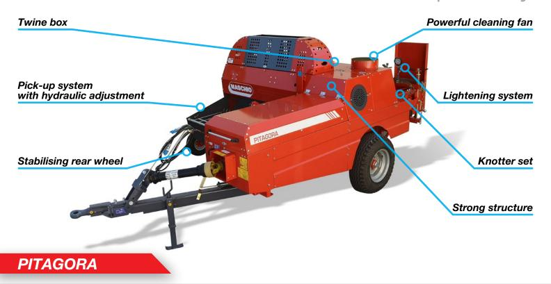
A versatile machine, reliable and easy to use. The bale results are very consistent and easily separate into flakes to simplify the hand-feeding operations. The standard fan keeps the knotter system clean in all conditions, the gear-driven knotter quality and design will ensure easy use and cut machine downtime.
