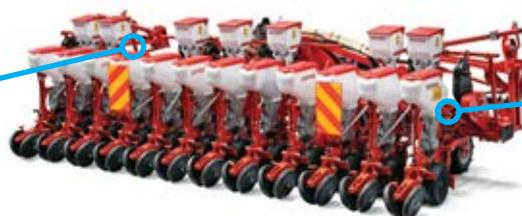
Hydraulically operated stack-folding side wings
