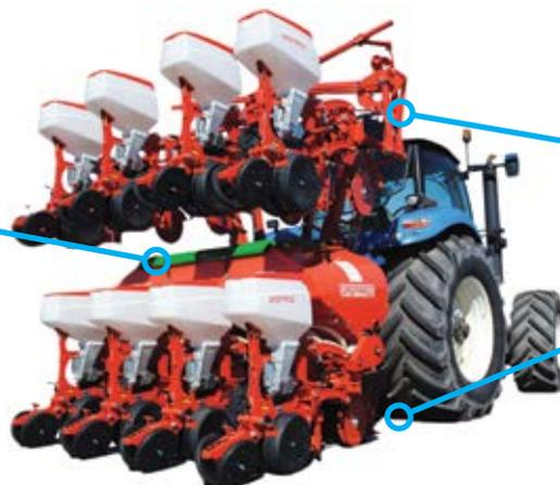
Hydraulically operated stack-folding side wings
