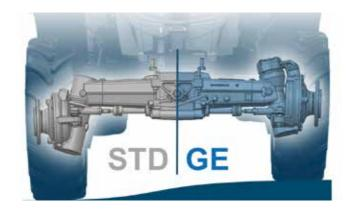
**MISTRAL2 GE, SPECIALISED IN LOW-CLEARANCE OPERATIONS** Specially designed for work in vegetable growing farms, greenhouses, vineyards and orchards grown on overhead trellis systems, the Mistral2 comes fitted with 20" and 24" rear tyres for maximum traction and stability. The front and rear axles of the Mistral2 GE are respectively 100 mm and 95 mm lower than on the Mistral2 STD.
