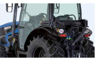
**CAB AND FRONT SUSPENSION FOR CONVENIENT OPERATION** The cab is mounted on a Hydro silent block suspension system or optionally on spring-type shock absorbers allowing a vertical travel of up to 60 mm. For the F, S and GT models a suspended front axle is available to effectively reduce vibration levels and enhance ride comfort.
