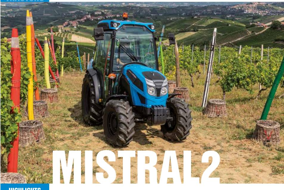
The Mistral2 is designed to combine superior performance with respect for the environment. Nimble and lightweight, this tractor provides excellent manoeuvrability and reduced soil compaction, making it ideal for vegetable farming, greenhouse operations and overhead trellis systems. Due to its agility, the Mistral2 is equally at home in orchards, vineyards and municipal applications like maintenance of green areas.
