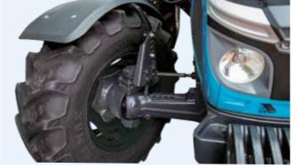
**RELIABLE AXLE PERFORMANCE IN THE FIELD AND ON THE ROAD** The **Powerfarm** features a braked front axle with differential lock and electrohydraulically engaged four-wheel drive. Wet multi disc brakes are fitted to ensure efficient braking on all four wheels. A high ground clearance and a 55-degree steering angle make for excellent manoeuvrability.
