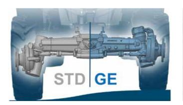
**SERIE 2 GE. SPECIALISED IN LOW-CLEARANCE OPERATIONS** The Serie 2 GE is specially designed for working in vegetable farms and greenhouses as well as in vineyards and orchards grown on overhead trellis systems. For this reason, both the front and rear axles are 100 mm lower than on the Serie 2 STD. The Serie 2 GE comes fitted with either 20" or 24" rear tyres for maximum traction and stability.
